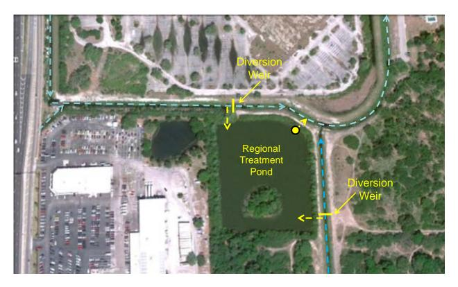
Figure 5-6. Conceptual Schematic for Regional Treatment Pond for Upstream Portions of Long Branch Creek.
