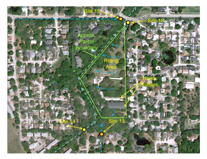
Figure 5-7. Overview of Drainage Patterns in the Vicinity of Main Channel Sites 14 and 16.
