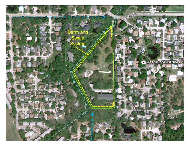
Figure 5-8. Proposed Berm and Swale System for Horse Stable Parcel.
