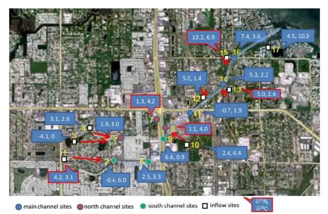
Figure 3. Map of Long Branch Creek and the sample sites, numbered 1-17. Red arrows indicate presumed flow from inflow stations to channel stations. Callout boxes show mean  $\delta^{15}$ N and  $\delta^{18}$ O values of nitrate measured for each site. Red outline indicates sites with average NO<sub>3</sub><sup>-</sup> concentrations > 0.2 mg N L<sup>-1</sup>
