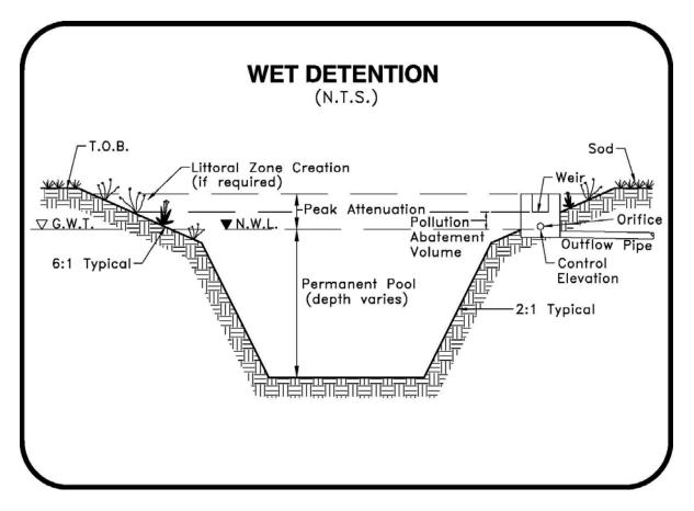
Figure 5-1. Schematic of a Wet Detention System.
