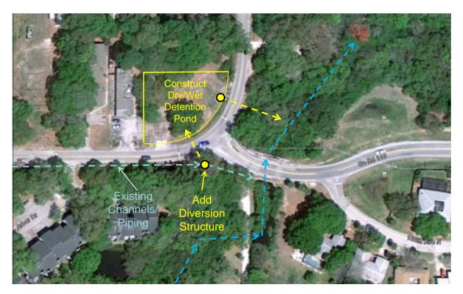
Figure 5-12. Alternative Conceptual Treatment System for the Whitney Road Drainage Swale.
