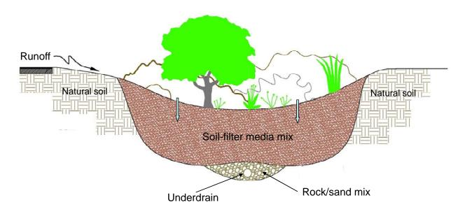
Figure 5-3. Modified Bio-retention System.
